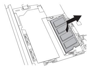
Figure 8-15 Removing the memory module
